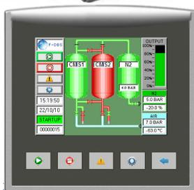
The generator is controlled using the latest in HMI touch screen technology to display the process in real time, inlet/outlet pressures and oxygen level (optional).
