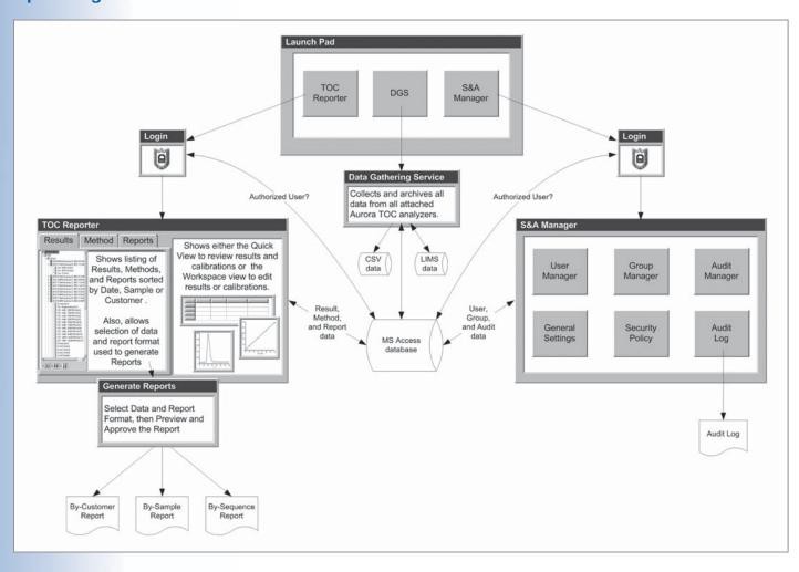
A schematic overview of A<sub>TOC</sub> software modules and their relationship to each other.
